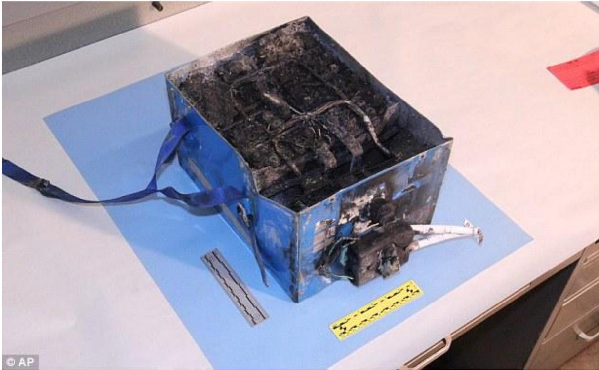
The Boeing 787's lithium battery can self-heat as a result of temperature and pressure changes, which may have caused this battery fire on the Dreamliner.
